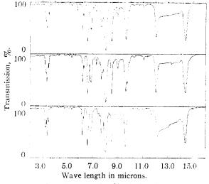
Fig. 2.—Infrared spectra of 10% solutions in carbon tetrachloride taken with a Baird double beam spectrophotometer with a sodium chloride prism: upper curve, 1-p-anisyl-1phenylethane from the decarbonylation reaction; middle curve, authentic 1-p-anisyl-1-phenylethane; lower curve, 1-p-anisyl-2-phenylethane.
