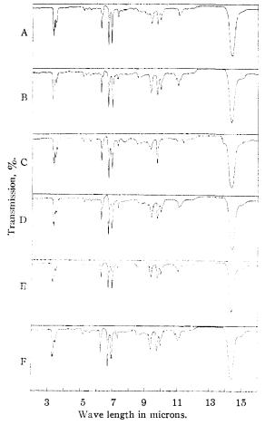
Fig. 1.—Infrared spectra of approximately 10% solutions in carbon tetrachloride taken with a Baird double beam spectrophotometer with a sodium chloride prism: A, 1,1,2triphenylpropane; B, 1,1,2-triphenyl-1-propene; C, 1,1,1-triphenylpropane; D, rearrangement product fraction 3; E, product fraction 1; product fraction 2.
